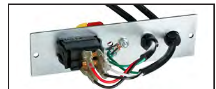
Figure 97. G1014Z switch wiring.
